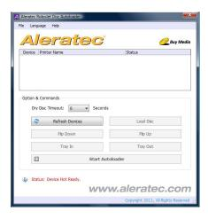
If this happens, please check that your printer and autoloader are installed correctly and being recognized properly by your computer. Once all the components are installed properly, click the "Refresh Devices" button to re-scan your computer's hardware.
